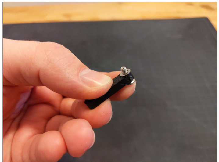
Step 108. Prep arm_A with m3x8mm bolt and a washer.
