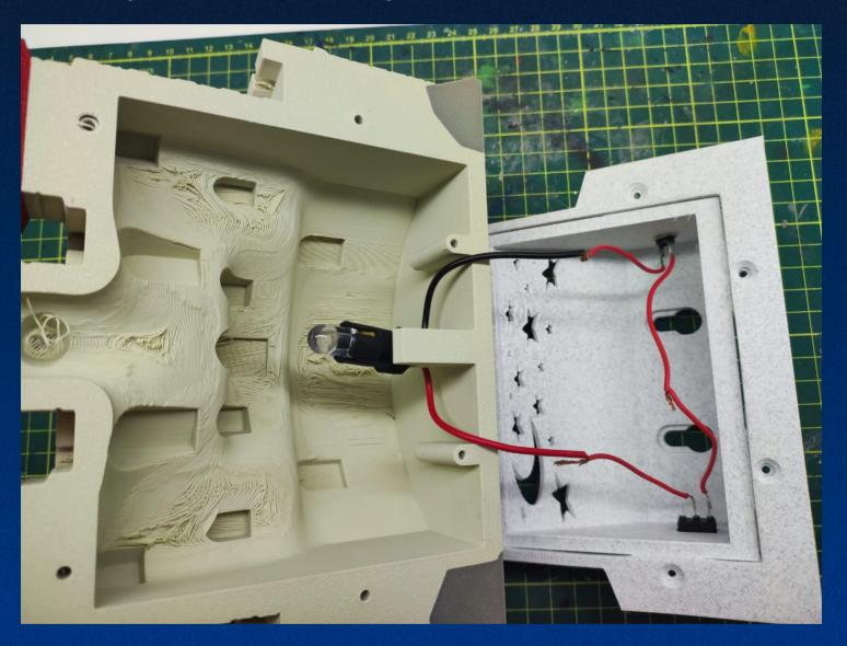
Put all the layers and the light body on the base and if need you can use screws to fix it all.
