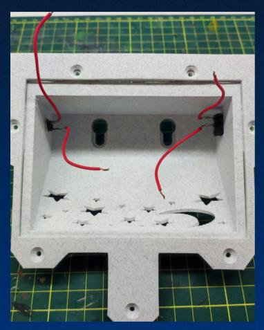
Solder the positive wire on one of the on/off switch's end.
