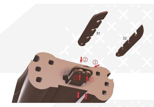
The assembly of the FDM version requires pins made out of short pieces of regular 1.75 mm filament.
