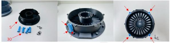
Pre-install 6 M3x8 Hex Screws as shown below: *Tip – There are holes to allow a screwdriver to access these Screws from underneath.*
