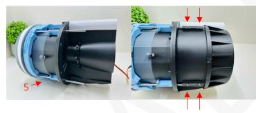
Slide Reverse Thrust Actuator to expose blocker door linkage mount. Insert Door Blocker Assembly into Reverse Thrust Door by inserting a pin first, then click the other pin: NOTE: You should hear a \*CLICK\*:
