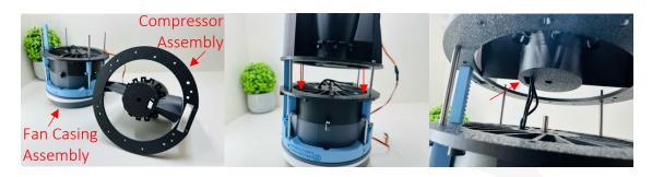
Secure using 8 M3x8 Hex Screws:
