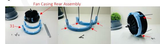
Insert 29 into Fan Casing Rear Assembly through the large rectangular slot from the rear. Slide 31 or 29 to line up the 4 M2x8 Hex Screws and fasten:
