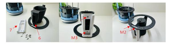
Secure the MG996R Servo into the Compressor Assembly using 4 M3x8 Hex Screws and route the wire down and through the larger hole of the Compressor Assembly. Ensure to orientate the servo correctly, a rectangular slot is for the Protruding Servo Wire:
