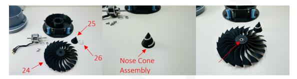
Secure the Nose Cone Assembly to 24 using 2 M3x8 Hex Screws ensuring M5 nut is inserted. Attach brushless motor Washer to the shaft. Attach Fan Assembly onto the brushless motor and tighten:
