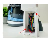
Once the program has been loaded on the Arduino, the reverse thrust actuator can be tested using the pushbutton. Some servo motors may be different so the angle may need to be adjusted slightly. You can test the pushbutton using USB power (without LiPo powering the Arduino).
