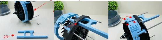
Slide the reverse thrust actuator back and forth and ensure it moves freely with minimal resistance.
