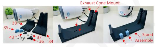
Assemble 36 & 37 using a single M3x8 Hex Screw. Press fit Thrust Lever to the potentiometer:
