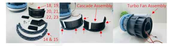
Secure both Cascade Assemblies to Turbo Fan Assembly using the 6 pre-installed M2x8 Hex Screws.
