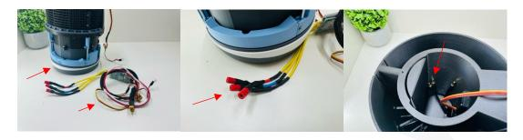
Secure ESC to Turbo Fan Assembly using the 20mm Velcro Strip utilising the rounded slot:
