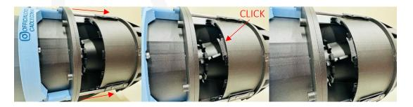
Attach Reverse Thrust Door Assembly to Turbo Fan Assembly and attach Door Blocker Assembly. Repat for remaining 11 Door Blockers.
