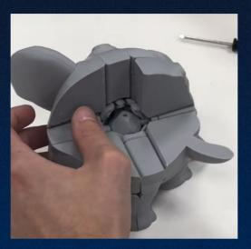
Screw the Center piece that was left unscrewed on step one to finish the mechanism assembly. Tight or loose the screws for better movement.
