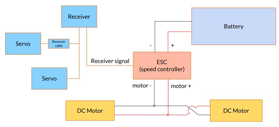
Rear motor must be connected in reverse!
