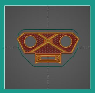
You can print Front Mask with filament changes to achieve color results. Please, setup filament changes in layer heights described below (setup is for layer height 0,15mm):
