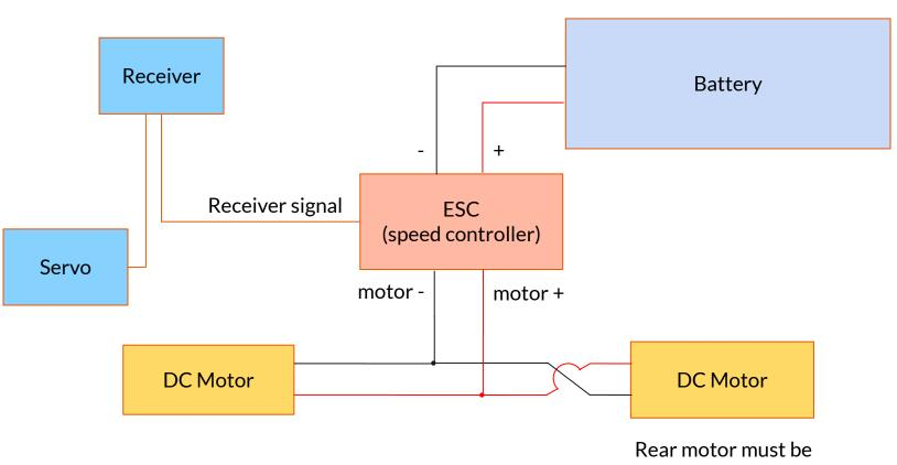
Rear motor must be connected in reverse!
