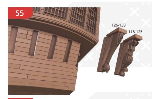
There are two versions of the corbels: a simplified version for FDM printing (parts #126-133) and an original version for SLA printing (parts #118-125).
